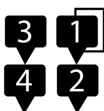
This algorithm splits the chain into a pair of 2op synths that can be detuned using the tune fader. Operator 4 is a carrier modulated by operator 3, and operator 2 is a carrier modulated by operator 1.
