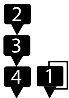
Operator 1 is left unmodulated, but applying vibrato with the op2 fader will cause it to bend. Operators 2-4 are set up similarly to Algo1. Operator 4 is the carrier and is modulated by operator 3, which is in turn modulated by operator 2.
