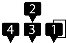
Operators 1 and 4 are carriers with no operators modulating them, while operator 3 is a carrier modulated by operator 2.
