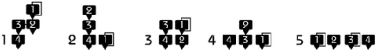
Synth voices consist of up to four oscillators called operators. If we observe the algorithm icons, the numbered boxes represent the operators and the arrows represent the modulation signal path.
