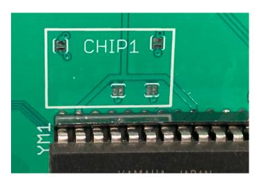
Following the instructions printed under the circuit board we simply add some solder across the 4 jumper pads to activate YM2612 mode and remove the solder to re-activate the default YM3438 mode.
